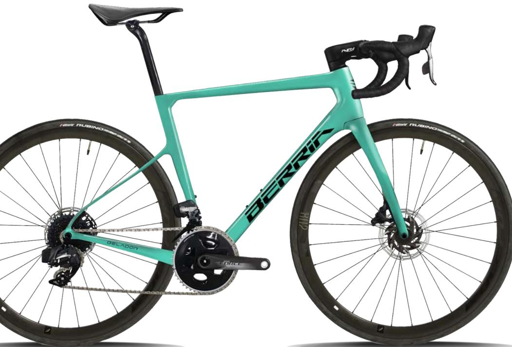
Belador Blade 5 full carbon fork, internal cable system ICS2, 1-1/8" - 1-1/2"
