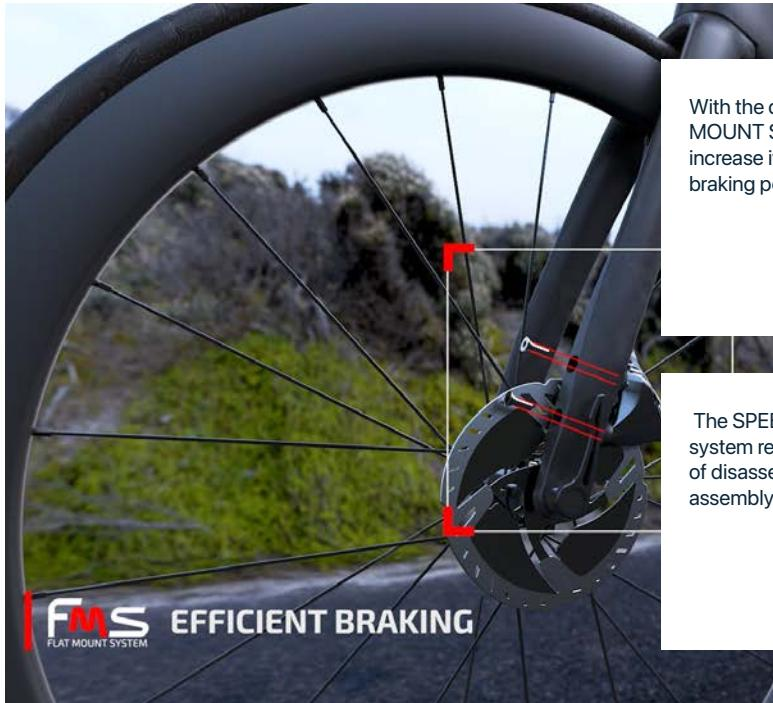
With the direct FLAT MOUNT SYSTEM we increase its rigidity, and braking power.
